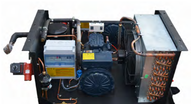
Compressors - Condensers - Fan - Selenoid Valves
